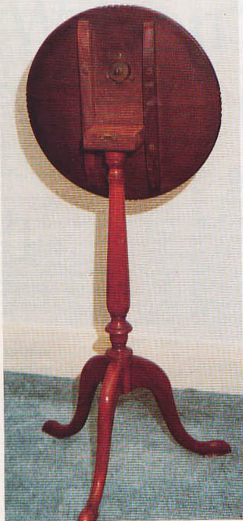
The bearers are attached across the grain to counteract any tendency for warping
