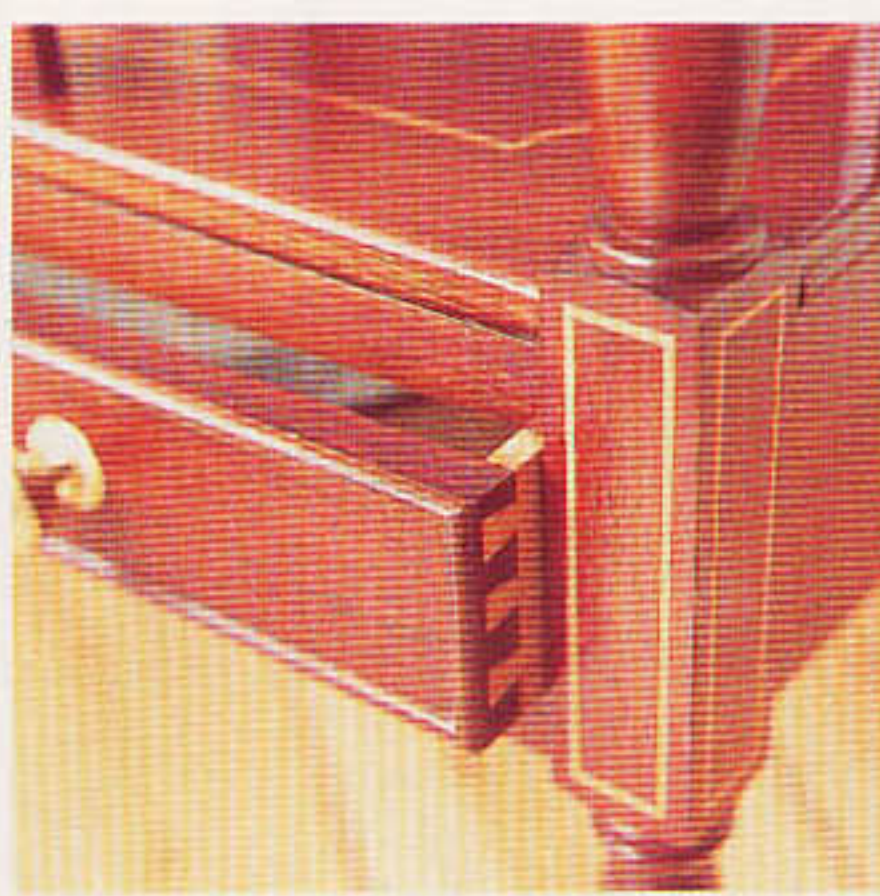
The drawers are of traditional lapped-dovetail construction with oak sides, back and bottom
